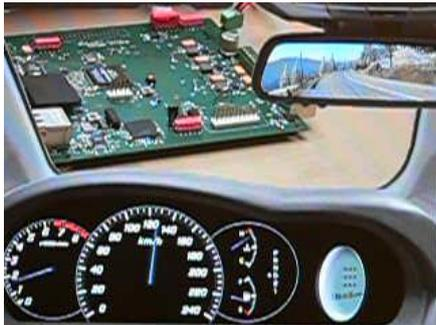
The BADGER kit includes HW and SW. The hardware consists of a PCB, sample display, power supply and cables. The board is delivered with an evaluation version of BADGE loaded in the FPGA. On power-up a standard demo is started. This gives the design team a flavor of BADGE's potential.
